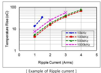
2) The rise in increase by self-heating of MLCC must not exceed 20°C
