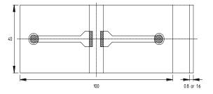
(Substrate for bending strength test)
