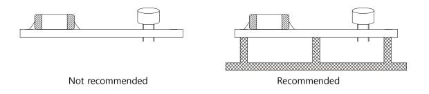
4-10-4. Socket and / or connector attach / detach
