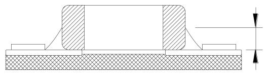
\* Soldering wire below ø0.5mm is required for soldering.
