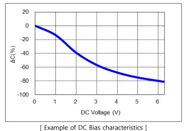
\* Sample : X5R 10uF, Rated voltage 6.3V
