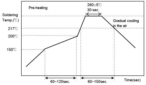
[Reflow Soldering Conditions]
