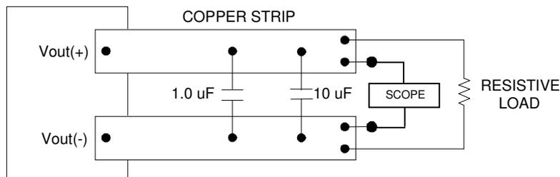
Note: Use a 1 $\mu$ F X7R ceramic capacitor and a 10 $\mu$ F @ 25V ceramic capacitor. Scope measurement should be made using a BNC socket. Position the load 3 in. [76mm] from module.
