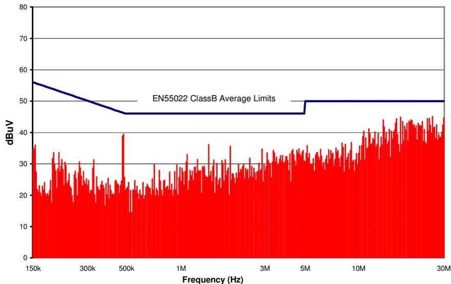
Figure 16. CPT20A48 Conducted Emissions using above specified input filter.
