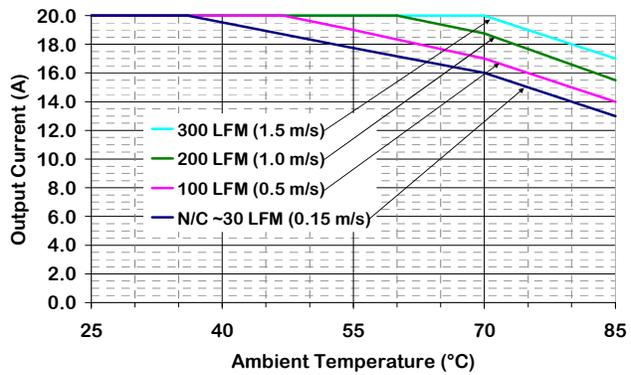
Figure 4. Output Current Derating vs Ambient Temp (converter mounted vertically with air flowing from pin 3 to pin 1, Vin = 48 Volts, with baseplate)
