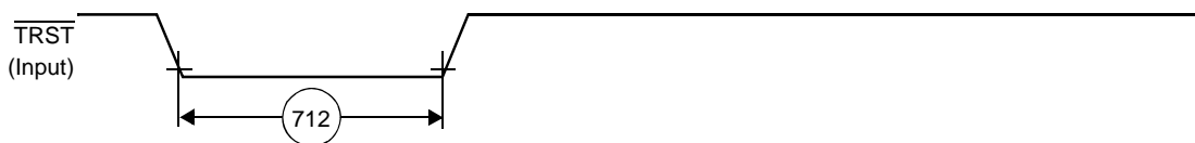
Figure 25. \overline{\text{TRST}} Timing Diagram
