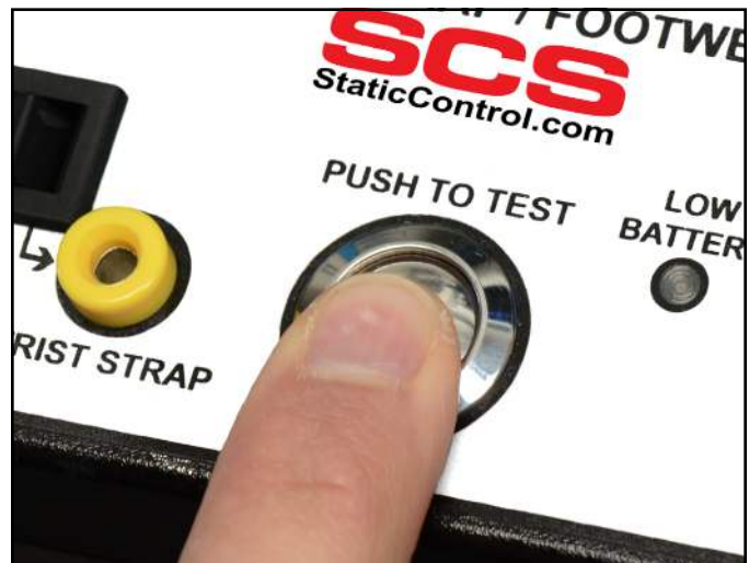
Figure 13. Bridging the pushbutton and its surrounding metal ring when performing a test
