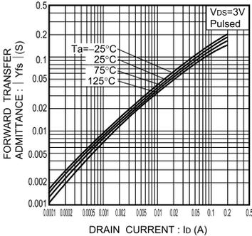
Fig.8 Forward Transfer Admittance vs. Drain Current
