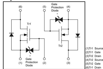
\* A protection diode has been built in between the gate and the source to protect against static electricity when the product is in use. Use the protection circuit when rated voltages are exceeded.
