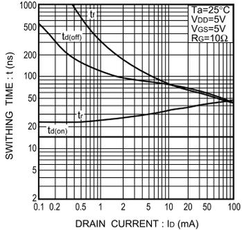
Fig.12 Switching Characteristics
