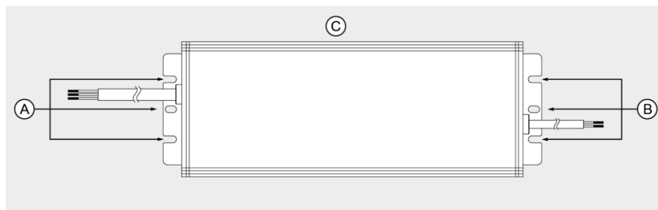
Fig. 3 Mounting Hole Locations
