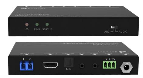
The TL-FO2-HDC2 is an HDMI 2.0 (18G signal) with HDCP 2.2 support fiber optic extender that can reach up to 300 meters (984 ft) over a duplex OM3 or OS2 cable with common LC terminations. The unit supports HDMI video resolutions up to 4K@60, HDR video, IR or RS232 pass-through controls, multichannel audio, as well as ARC with optional optical audio embedding and/or de-embedding. The TL-FO2-HDC2 is also compatible with HDMI 1.3/1.4 content with HDCP 1.3/1.4 content protection.
