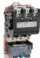
Non-reversing motor starter Size 4 Three phase full voltage Solid-state overload relay OLRelay amp range 50-200A 550/575-600 50/60HZ coil Combination type No enclosure
