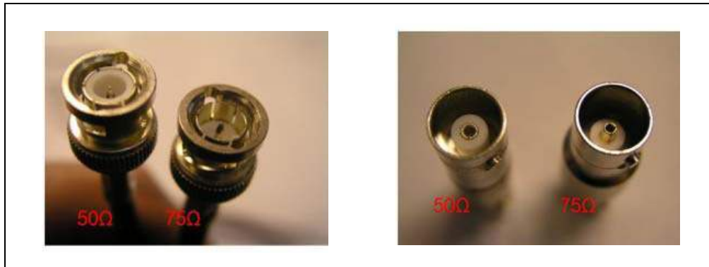
FIGURE 1-4: DIFFERENCE BETWEEN 50\Omega VS. 75\Omega CONNECTORS
