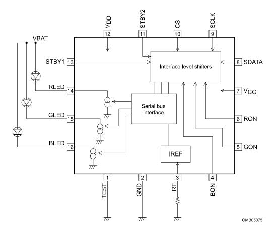
Note 1: The TEST pin must be tied to ground.
