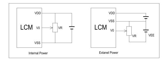
V<sub>DD~</sub>V<sub>0</sub>: LCD Driving voltage
