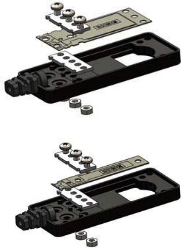
Figure 73: Clamping the piezo products is possible with three recessed nuts, three low profile M3 bolts, two clamp plates (-6mm PPA-5005 shown) and the PPA-5008 clamp enclosure base. Left: PPA-X014. Right: PPA-X022.
