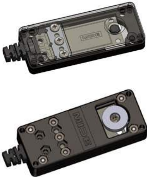
Figure 74: Left: Enclosure clamp base with thinner clear top paired with tactile bumper. Right: Enclosure clamp where two “bases” are used to create an enclosure.
