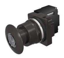
30mm BlackMax, Epoxy Coated Corrosion Resistant Complete Metal Unit Illuminated Push-Pull Operator Transformer type, 120V AC LED Lamp Mushroom Head Cap Small 1 3/4" (44.5 mm) Metal, Black with Clear Lens 3 Position Pull-Momentary/Push-Maintained UL Listed, CSA Certified NEMA 1,3,3R,4,4X,12,13 & Automotive Standards
