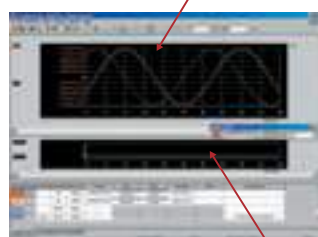
The traced waveforms can be displayed as layers. Sampled value from a specific input bit will be displayed.
