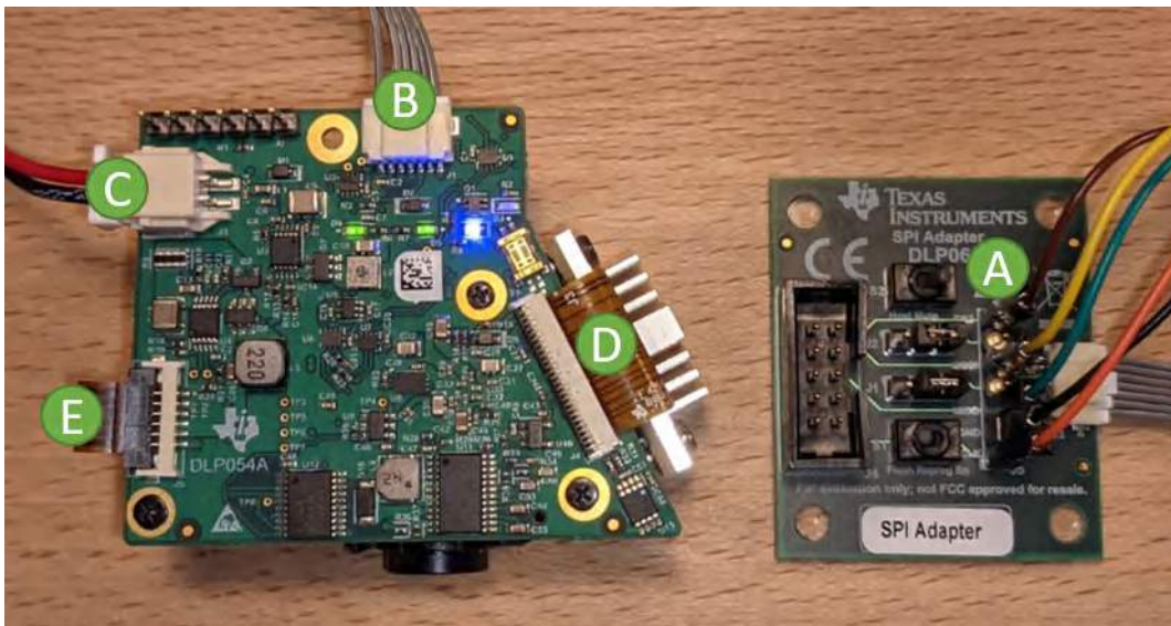
Figure 3-2. Assembled DLP3021-Q1 Light Engine EVM with FTDI
