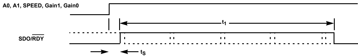
FIGURE 28. \overline{\text{SDO/RDY}} DELAY AFTER MULTIPLEXER CHANGE
