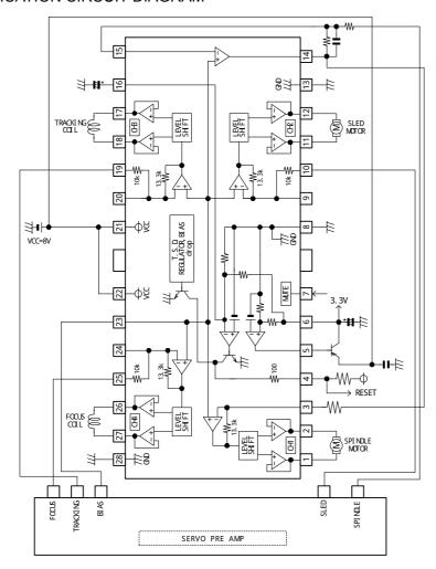
CH1: SPINDLE CH2: SLED CH3: TRACKING CH4: FOCUS
