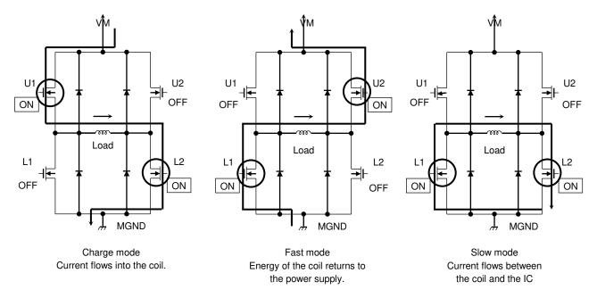
\*When the output switches, cross-conduction protection time is provided in the IC to avoid penetrating current.
