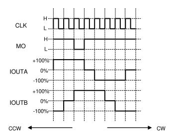
Waveform of MO output: State of pull-up.
