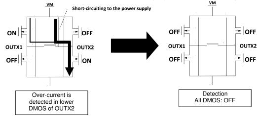
•When over-current is detected in the lower DMOS of H-bridge by the short-circuiting to the power supply:
