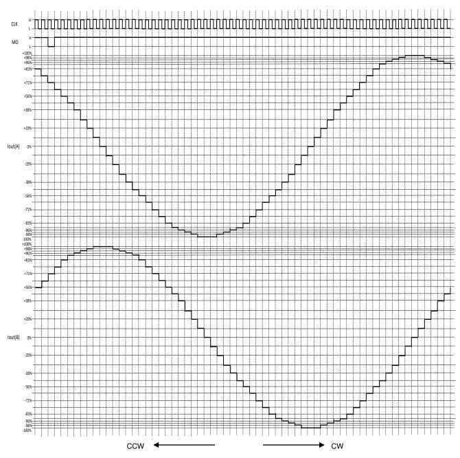
Waveform of MO output: State of pull-up.
