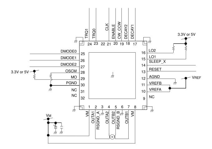
Heat dissipation PAD (4 corners and the center part) on the back of the package is recommended to connect to the GND of the board for improved heat dissipation.
