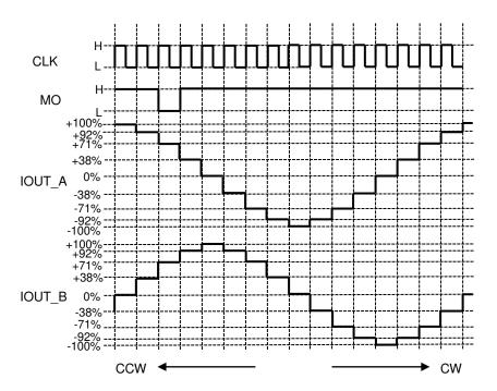
Waveform of MO output: State of pull-up.
