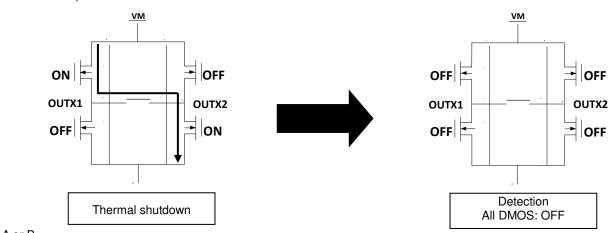
•When over temperature is detected:
