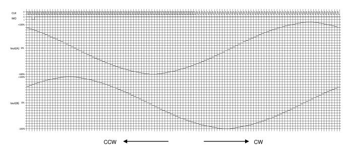
Waveform of MO output: State of pull-up.
