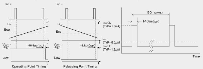
This Hall effect IC's output is held as internal data just before the internal circuit turns OFF (loo OFF). And after 48.8  $\mu$ s, the output changes.
