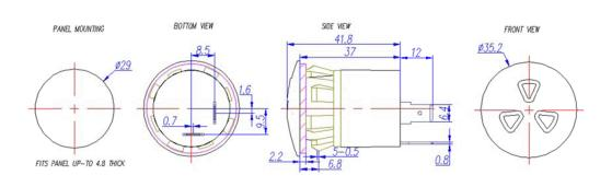
General tolerance = ±0.75 mm and all measurements in mm unless otherwise noted.
