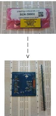
b) Next, break header strip (included in pacakge) into segments properly sized for an Arduino Uno R3 Shield install. This gives a 6, 10 and two 8-pin segments. The ICSP header is NOT used with this shield
