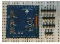
Note: Pins required for this board are as follows Uno R3 Layout SCL and SDA (I2C comm) Power: 5.0V, 3.3V, and all GND pins Pushbuttons: D9, D7, D5 LEDs: D8, D6, D4
