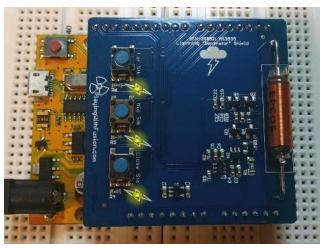
h) You're ready to use the emulator! Place the AS3935 antenna somewhere between 4 and 10 cm from the inductor on the emulator board. Pressing the buttons will emulate far, mid-range and near lightning strikes, giving different absolute readings and distance estimates from the lightning sensor. The LEDs next to the button you just pressed should light for approximately 1 second.
