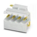
PCB headers, color: light grey, contact surface: Gold, contact connection type: Pin, number of rows: 1, number of positions: 4, product range: MSTBO 2,5/..-G1L Au, pitch: 5 mm, mounting: Wave soldering, pin layout: Linear pinning, solder pin [P]: 3.5 mm, number of solder pins per potential: 1, plug-in system: COMBICON MSTB 2,5, Pin connector pattern alignment: Orthogonal, locking: without, type of packaging: packed in cardboard, Product with pin output on left side
