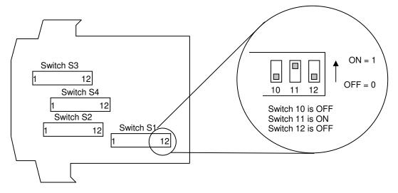
Switch S1 and S2 configure the input type and range, and switch S3 and S4 configure the output types, ranges and a few additional functions. The switch settings are explained in the next few pages. The diagrams refer to switch positions 0 and 1, with 0 being OFF and 1 being ON. This is illustrated in the picture above.
