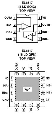
\*THERMAL PAD MUST BE CONNECTED TO NEGATIVE SUPPLY:  $V_S$ -QFN PACKAGE CAN BE USED IN DUAL SUPPLY APPLICATIONS.
