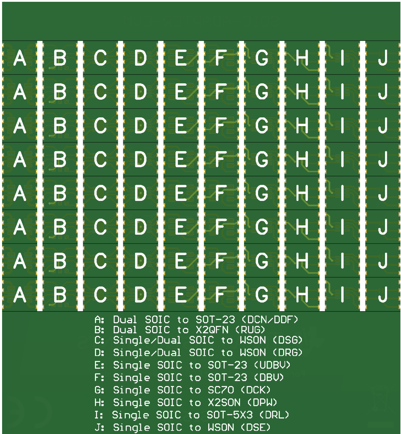
Figure 4-2. PCB Bottom Layer
