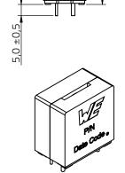
Pin 2 and 3 are only for mechanical stability.
