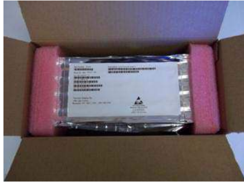
Figure 39. Brick Loaded in Shipping Container
