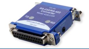
Model 422LCOR, non-isolated RS-232 to RS-422 converter, converts unbalanced RS-232 signals to balanced voltage digital interface to allow communications of 90K bits per second on cable lengths of 1200 meters (4000 feet). Ten receivers can be connected to any one driver for use in multi-drop systems.
