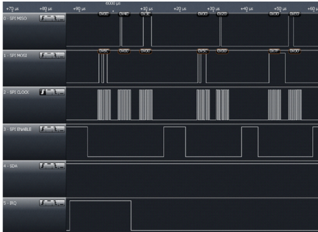
Figure 6-24. IRQ With One Byte in FIFO
