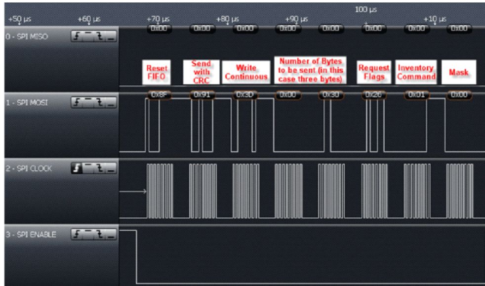
Figure 6-20. Inventory Command Sent From MCU to TRF7962A
