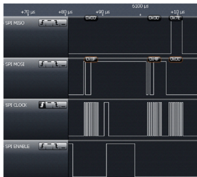
Figure 6-25. Reset FIFO and Read RSSI
