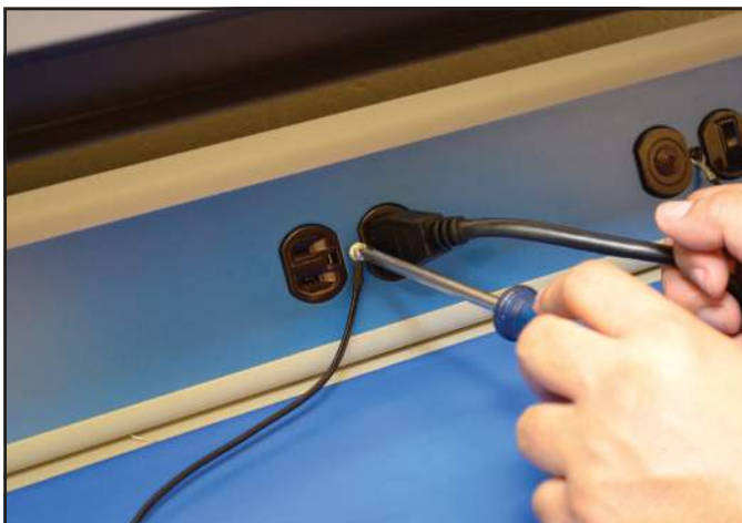
Figure 8A. Attaching system grounds. Note work, surface and unit are grounded at different locations.
