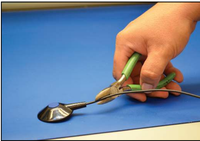
Figure 7. Cutting off table mat ground snap.
