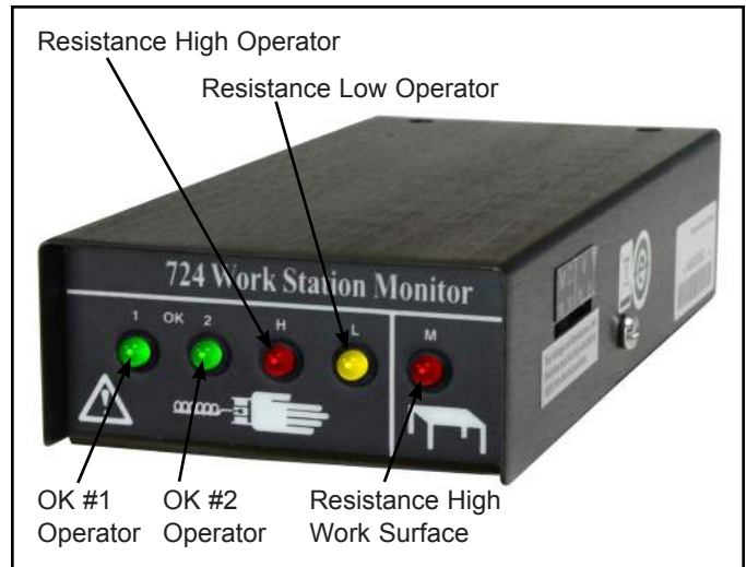
Figure 4. SCS 724 Workstation Monitor features and components
