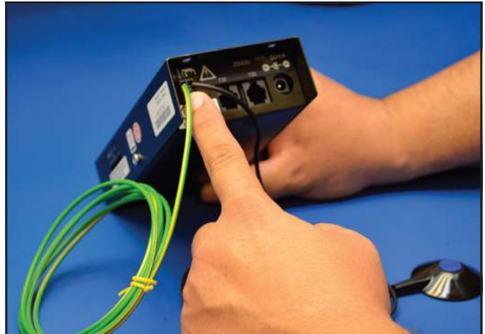
Figure 9. Inserting two-wire connector into rear of SCS 724 Workstation Monitor
