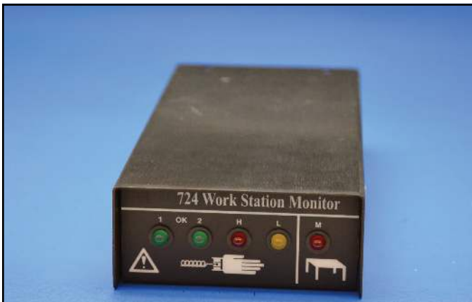
Figure 11. SCS 724 Workstation Monitor mounted on benchtop.
