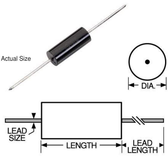
**Mechanical Configuration** Units are axial leaded for thru-hole mounting, encapsulated in an epoxy molded case. High resistivity ferrite core, allows for high inductance with low DC resistance.
