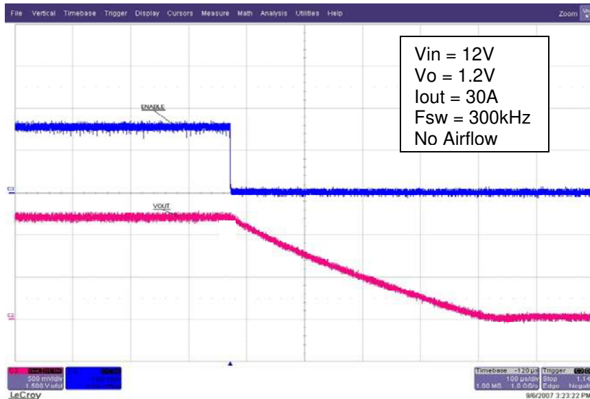
Fig. 8: Close-up of Power Down when Enable is pulled low
