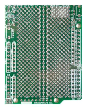
Through Hole Prototyping Shield for Arduino Uno with Components and Free Breadboard
