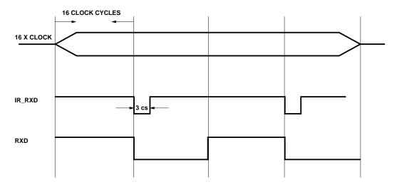
A high to low transition of the IR\_RXD line from the infrared transceiver module signifies a 3/16th pulse. This pulse is stretched to accommodate 1 bit time (16 clock cycles). Every
