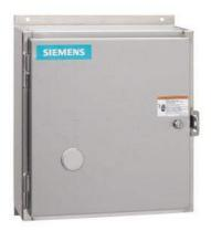
Non-reversing NEMA contactor, Size 4, Three phase full voltage, Contactor amp rating 135A, 3 wire (NO aux included), 240V 50Hz / 277V 60Hz coil, Non-combination type, Encl NEMA type 4X 304 S-Steel, Water/dust tight noncorrosive, Extra-wide enclosure
