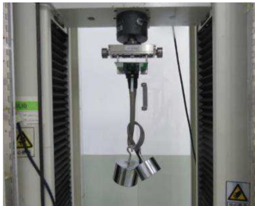
Figure 2 – Latch retention Test Setup
