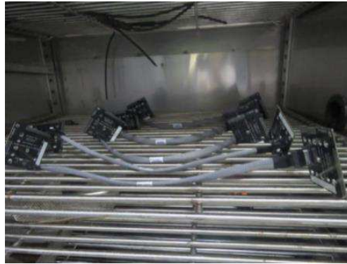
Figure 9 – Damp Heat Steady State Test Setup
