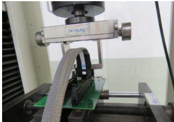
Figure 6 – Mating Force Test Setup
