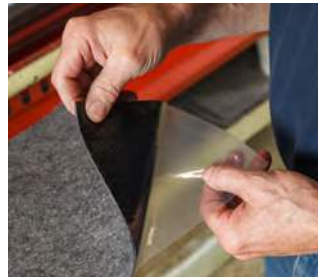
Permanent adhesive mat is protected by clear liner that must be removed prior to use.
