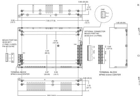
B: MOUNTING HOLE 8 PLACE 6-32 UNC(Zn-plated) SCALE 4:1
