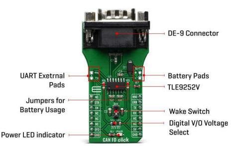
The CAN FD Click supports five different Modes of operation. Each mode with specific characteristics in terms of quiescent current, data transmission or failure diagnostic. For the mode selection the digital input pins EN and STB are used.
