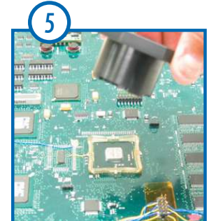
5 Lift to remove the Knob Tool - leaving the Frame Clip attached to the component.
