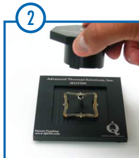
2 Position the Knob Tool over the Frame Clip
