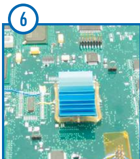
6 Place the Heat Sink squarely in the Frame Clip over the component. Note the direction of air flow when placing your Heat Sink.
