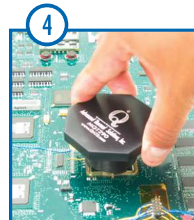
4 Position the Knob Tool with Frame Clip over the component, rotate 45° counter-clockwise releasing the Frame Clip
