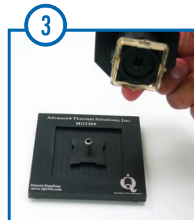
3 Rotate the knob tool 45° clockwise locking the Frame Clip to the Knob Tool and lift away from base plate.
