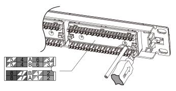
2. Punch down solid cable to each port until termination is completed.
