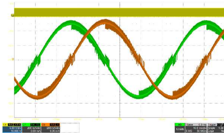
Figure 8-7. 1/256 Microstepping With smart tune Ripple Control Decay
