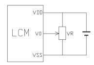
VDD~V0: LCD Driving voltage
