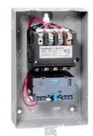
Non-reversing motor starter Size 1 3/4 Three phase full voltage Solid-state overload relay OLRelay amp range 10-40a 220-240/440-480VAC 60HZ coil Combination type Indoor general purpose use
