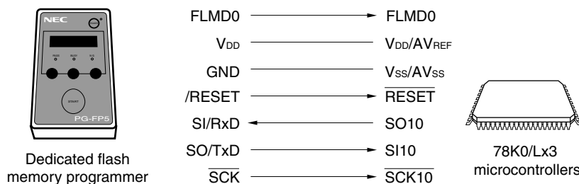
Figure 28-4. Communication with Dedicated Flash memory programmer (CSI10)
