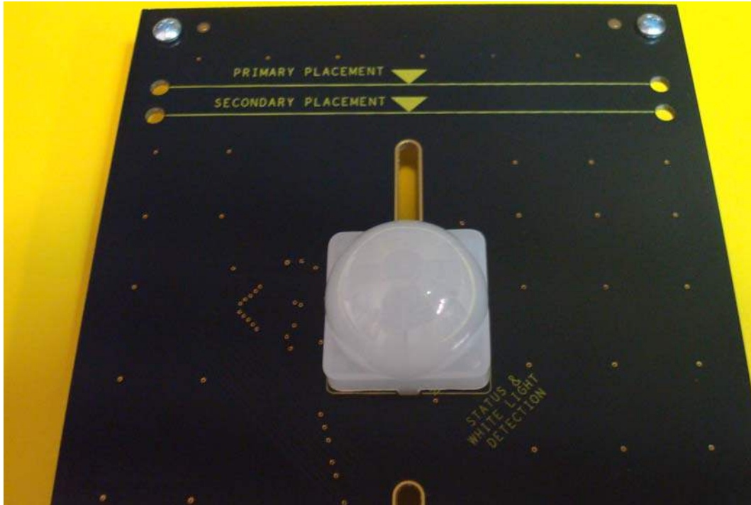
Figure 2. Assembled Clip-In Lens Installed on the ZMOTION 20-Pin Detection and Control Development Board
