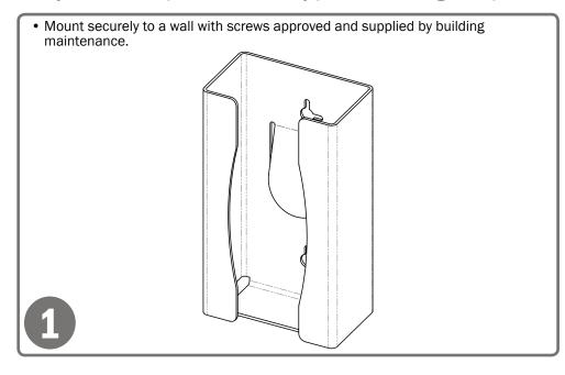
Dispenser can be mounted onto a BOWMAN<sup>®</sup> door or wall hanger through the cutout in the back. Care and Construction Stainless Steel
