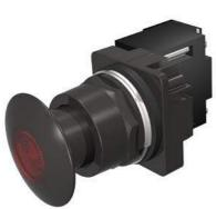
30mm BlackMax, Epoxy Coated Corrosion Resistant Complete Metal Unit Illuminated Push-Pull Operator Transformer type, 240V AC LED Lamp Mushroom Head Cap Small 1 3/4" (44.5 mm) Metal, Black with Red Lens 3 Position Pull-Momentary/Push-Maintained UL Listed, CSA Certified NEMA 1,3,3R,4,4X,12,13 & Automotive Standards
