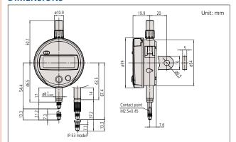
Note 1: Dimensions of the inch (ANSI/ AGD Type) dial indicator partly differ from those of the metric (ISO/JIS Type) indicator.
