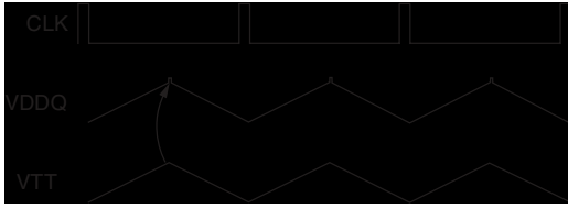
Figure 8. Noise-susceptible In-Phase operation for DDR2
