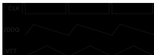
Figure 7. Optimal In-Phase operation for DDR1
