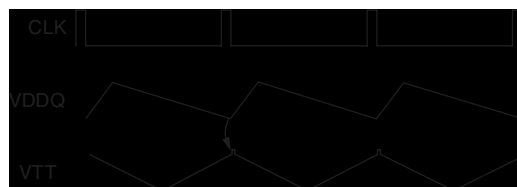
Figure 6. Noise-susceptible 180° phasing for DDR1
